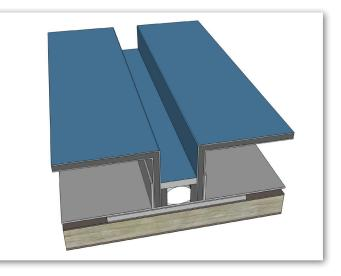
After panels are installed, rather than caulking, high-bond tape & silicone sealant are applied to the joint along with a color matched filler strip (see picture). This system has a typical overall depth of 1.5/8" and standard joint width of 3/4".
