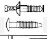
Chrome pin rivet has high shear strength but should be used in low moisture areas. Installation is the same as plastic pin rivet above.
